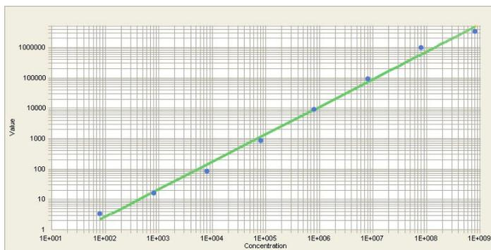
Figure 2. Europium standard curve. The calculated correlation coefficient of the curve is 0.9945
