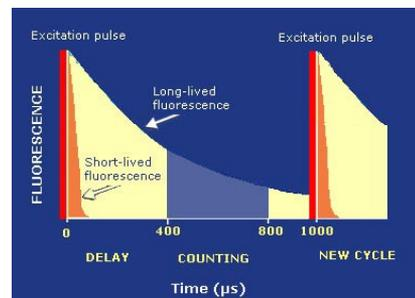
Figure 1. Basic principle of time-resolved fluorescence measurement. The excitation is made by very short light pulses and the emission is detected after a certain delay. The integration (counting) time in the figure is 400-800 µs.
