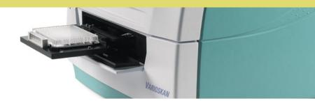
This technical note describes how to perform the basic time-resolved fluorescence measurements with Thermo Electron's Varioskan spectral scanning multimode reader and Skanlt software. The procedures of endpoint, scanning and decay time measurements are described using europium as a pattern fluorochrome.
